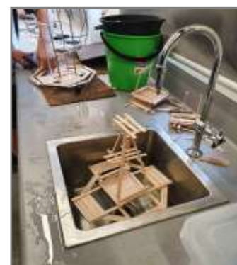
STEM Structural Engineering Challenge: Students applying principles of buoyancy, ballast and centre of gravity to design floating oil rig platforms.
